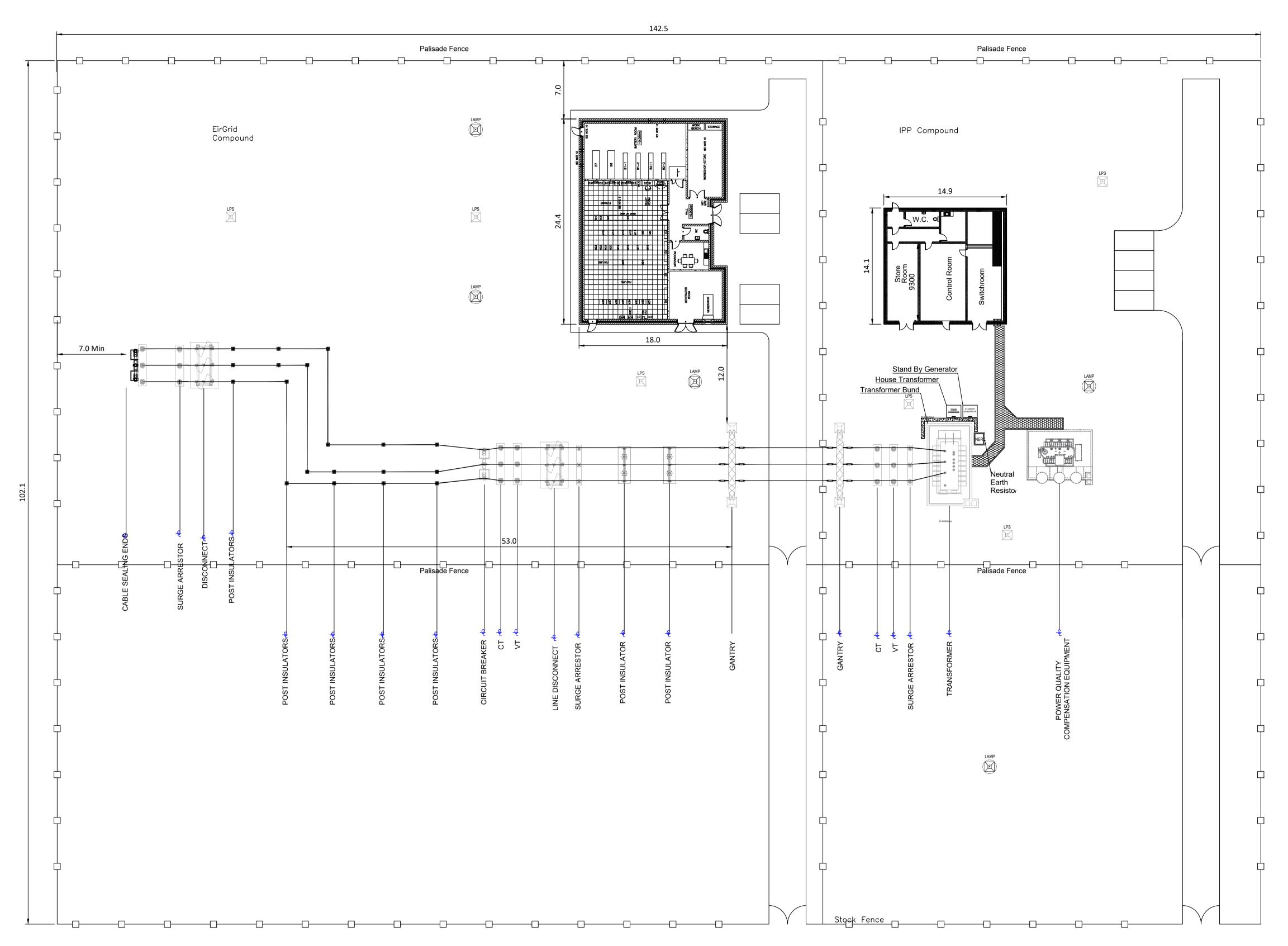
Legend LIGHTING MAST SURGE ARRESTER VOLTAGE TRANSFORMER CURRENT TRANSFORMER, SINGLE PHASE POST INSULATOR LINE TRAP (TYPICALLY R & T PHASES) LINE/EARTH DISCONNECT TRAFO/EARTH DISCONNECT CIRCUIT BRAKER BUSBAR DISCONNECT SA1/SA2 SB1/SB2 SECTIONALISER DISCONNECT
